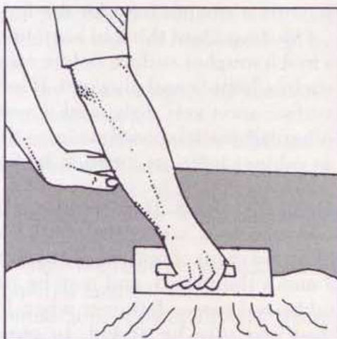
4. Apply mastic, then install tile or roll flooring.
